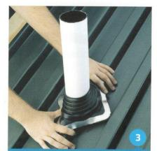
Press Master Flash\* down, bending it to conform to roof profile or roof irregularities. A blunt tool will help press the flashing into tight roof angles.
